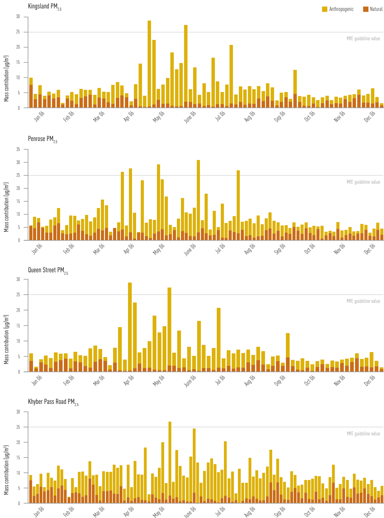
FIGURE 6 Seasonal variations in natural and anthropogenic sources of PM 2.5 particulates at monitoring sites in 2006. (Source: ARC).
