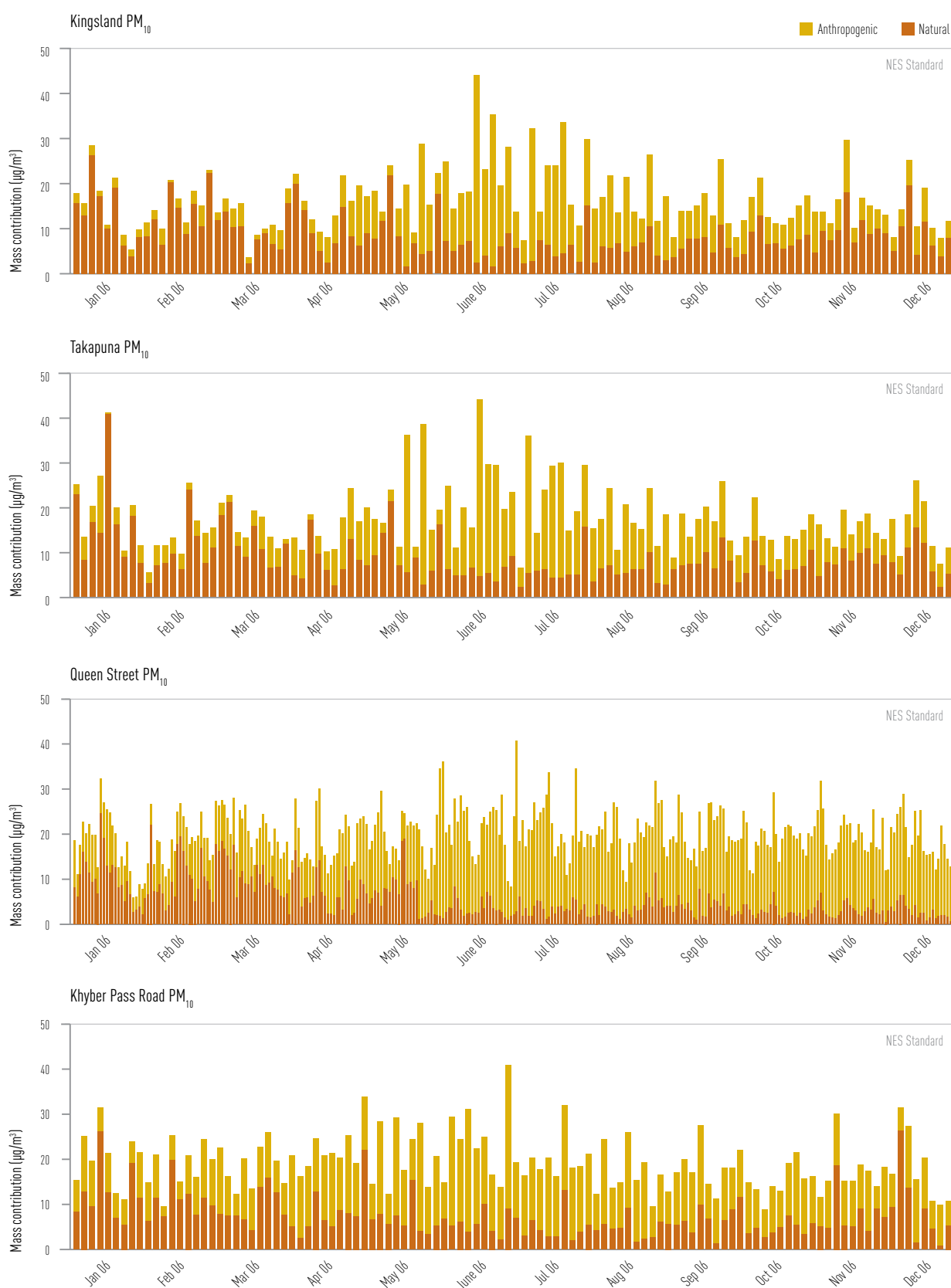
FIGURE 5 Seasonal variations in natural and anthropogenic sources of PM 10 particulates at monitoring sites in 2006. (Source: ARC).
